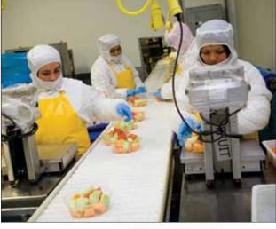
Fruit trays are being assembled and check-weighed within high-care facility before going to separate packaging area.
